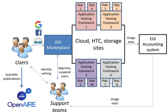
Fig. 1. The high-level overview of the EGI Applications on Demand service architecture.
