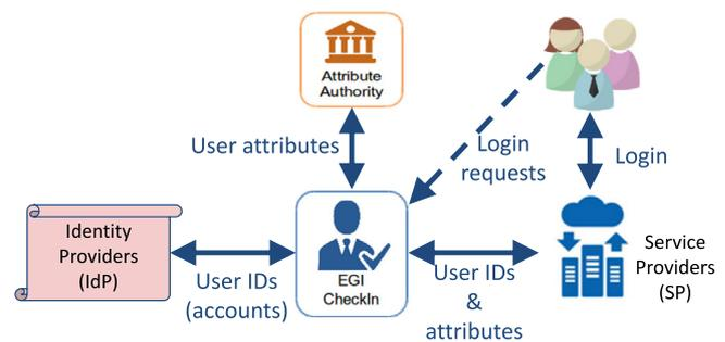
Fig. 2. The high-level architecture of the EGI AAI Check-In service.
